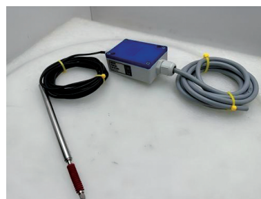
(b) Micro-Epsilon MSC7401 dedicated signal conditioner (Single-channel LVDT controller with IP67 protection, 8 units for signal processing)
