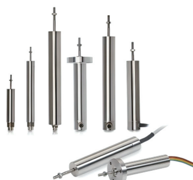
(a) Micro-Epsilon DTA-5G-3-CA inductive displacement sensors (resolution:0.001 mm, 8 sensors for center and edge measurement)
